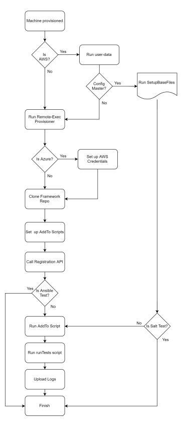
Fig. 4.3 Process of provisioning and testing by node type
