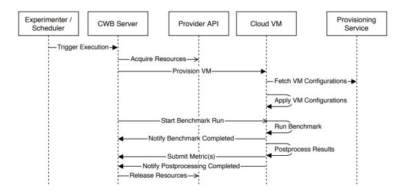
Fig. 2.3 Process Flow for CloudWork Bench tool (Scheuner and Leitner, 2019)
